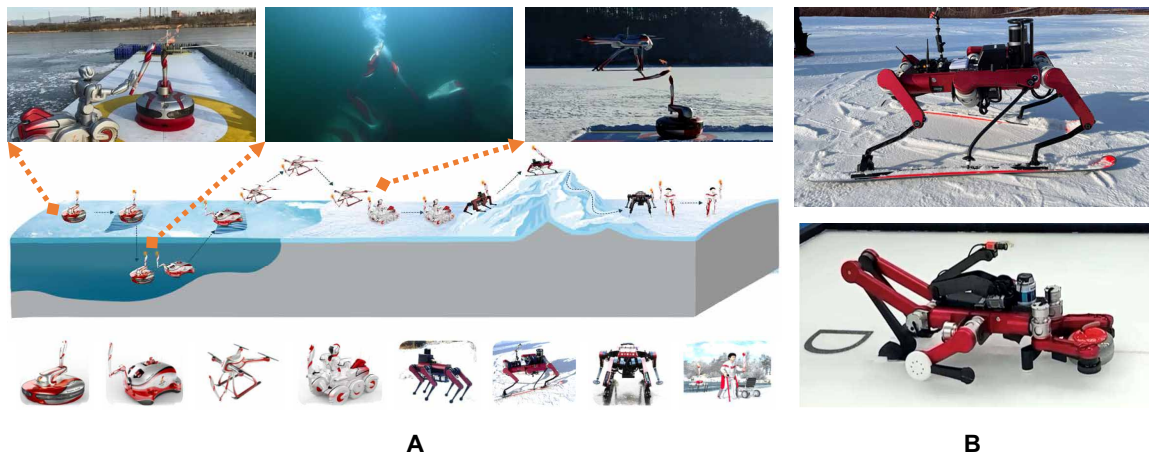
Fig. 1. Torch relay, skiing, and curling robots showcased during the Beijing 2022 Winter Olympic Games. (A) Robots developed for the torch relay involved ground, air, and underwater transfers. The amphibious robot and the underwater robot with variable structures were employed for the actual relay in the Beijing Winter Olympic Park, realizing the first underwater torch relay between robots in the history of the Olympic Games. (B) Top: Six-legged skiing robot. Bottom: Hexapod curling robot developed for Beijing 2022 Winter Olympics.
